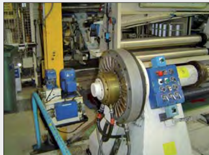
Konstanten Regelung an einer Druckmaschine Load closed loop regulation on a printing machine
