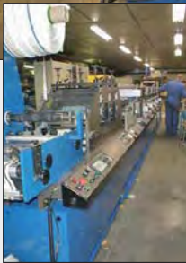
Zugregelung an einer Flexo-Druckmaschine Tension control on a flexographic printing machine
